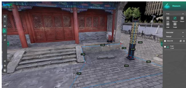
A powerful 3DGS measurement tool. It allows accurate distance, area, and angle measurements within photorealistic real-world 3D scene models, enabling users to obtain real-world spatial data directly in the browser—intuitive and efficient.
